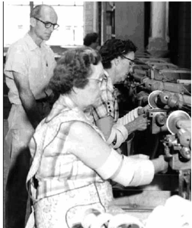
Figure 3—Finishing Asbestos Gaskets. Reproduced from: “Garlock 2009” Slide Presentation. Olwin Moeller v. Garlock Sealing Technologies, LLC . Case Number: 3:07-CV-65-H. United States District Court, Western District of Kentucky at Louisville.
